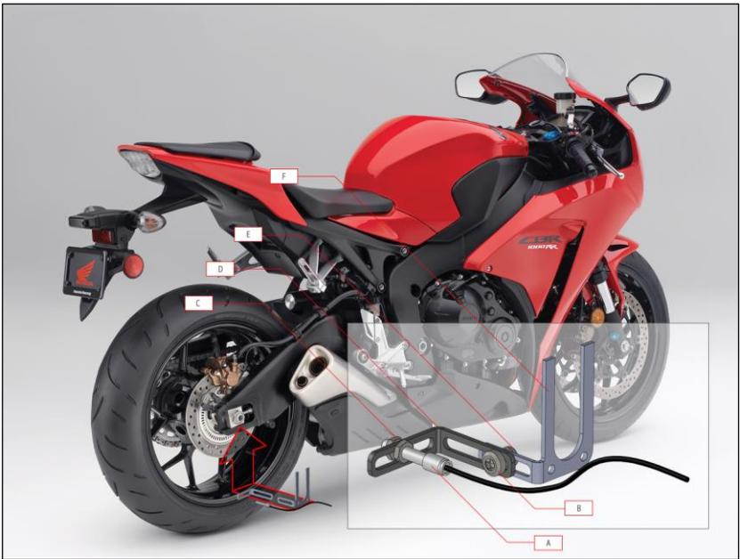
The rear brackets must be insert under the rear axle nut. Follow those step:
