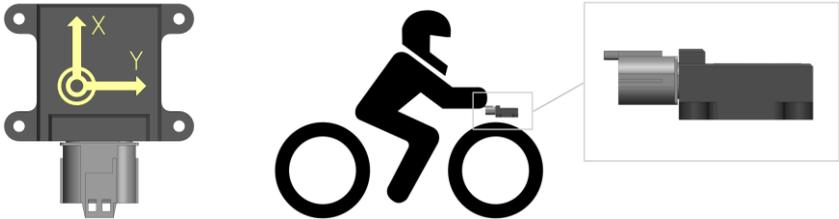
The GRIPONE IMU CAN may be sensitive to the vibration, for that reason we suggest to fix the body of IMU by rubber silent blocks. The best place of IMU is in the center of the front end of the vehicle. If the IMU is placed in the middle of the vehicle, it could not recognize the wheelie.
