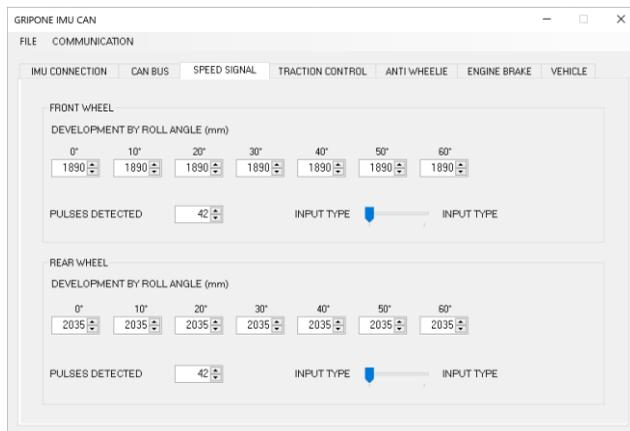
The development of the wheel is measured in mm. For each wheel there are seven fields where insert the development by the roll angle. The roll angle is zero when the vehicle is perpendicular to the ground.
