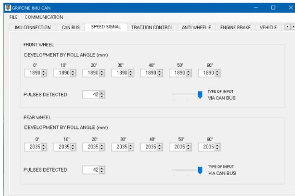
The development of the wheel is measured in mm. For each wheel there are seven fields where insert the development by the roll angle. The roll angle is zero when the vehicle is straight (perpendicular to the ground). The roll angle is 60° when the vehicle is leaned to the left or to the right side.
