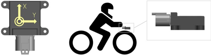
The GRIPONE IMU CAN may be sensitive to the vibration, for that reason we suggest to fix the body of IMU by soft rubber silent blocks. The best place of IMU is in the center of the front end of the vehicle. If the IMU is placed in the middle of the vehicle, it could not recognize the wheelie.
